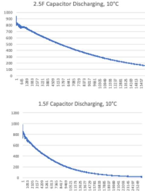
Figure 4. 2.5F (top) and 1.5F (bottom) Capacitors' Discharge Curves at 10°C, Samer Elhoushy<sup>b</sup>
