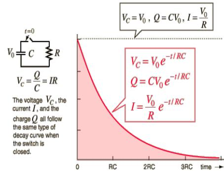
Fig. 2. Capacitor’s Charge and Discharge Formula and Curves, Images Courtesy of Hypherphysics
